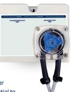
Keeping the pH of your pool water within the correct range is essential to ensure the sanitiser works efficiently. The pH system is available as a separate "plug-andplay" upgrade kit for the SWC 15, 25 and 35, with pH regulated via a separate peristaltic dosing pump (pictured). The pH dosing system is incorporated into the larger SWC 45 and SWC 60 control units.
